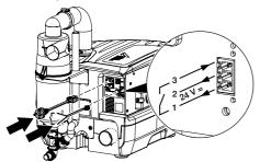
> Plug the network cable for the Tyscor Pulse into the network connection (optional when using Tyscor Pulse).
