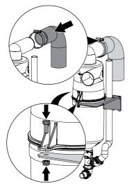
Attach the condensate separator with the holder to the unit and secure.
