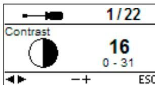
The cursor keys (79, 80) can be used to toggle between the possible settings. This screen can be left with the ESC key (71) or one of the program keys (82, 83, ...).
