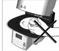
Never place objects in the hot firing chamber by hand, since there is a burn hazard. Always use the sinter tray fork supplied for this purpose. Never touch the hot surface of the furnace head, as there is a burn hazard. Please also observe the warnings on the furnace.
