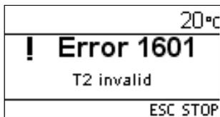
The furnace continuously monitors all functions during operation. As soon as an error is found, a corresponding error message will appear. In case of an error, the heater is switched off for safety reasons. The following error messages may be displayed:
