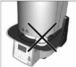
Sinter trays must not be placed in the area surrounding the firing plate, since this will obstruct the closing of the furnace head.
