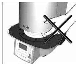
The furnace head is equipped with an electric drive and can be operated by means of the electronic controls. Never open the furnace head by hand, since this will damage the transmission.
