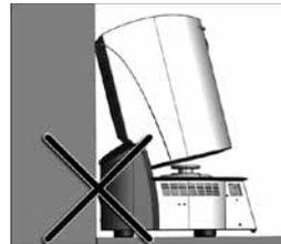
Do not use the furnace without spacer, since the distance to the back wall has to be kept!
