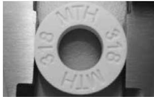
6. Find the measured diameter in the conversion table and read off the corresponding temperature. Only if the deviation is more than 10 °C must the furnace be readjusted.
