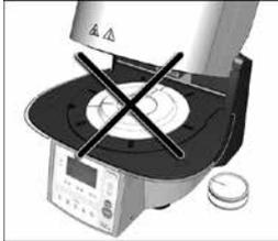
Never use the furnace without the sinter tray. Use only the original Programat sinter tray. Do not use the firing trays or honey-combed trays from conventional ceramic furnaces. Furthermore, check the sinter tray for damage, cracks or contamination before every program start. If the sinter tray is damaged, it must no longer be used. A maximum of one sinter tray is to be placed in the sintering chamber. Do not stack the sinter trays.
