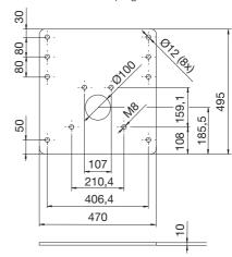
> Fix the unit to the wall mounting plate using four M8 screws.
