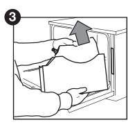
Remove the empty cleaning solution bag and discard or recycle it.
