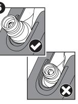
Ensure the nozzle is in the correct position.
