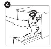
Connect the new bag, close the door and power the unit ON.
