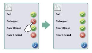
**NOTE:** The system can also be primed by simply starting a cycle and selecting "Detergent Replaced", when prompted.
