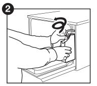
Disconnect the cleaning solution connector.
