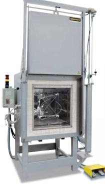
Holding frame for measurement of temperature uniformity
