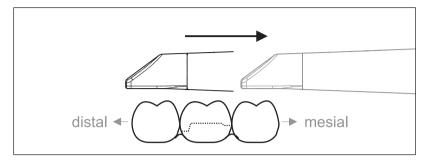
**Important:** Ensure that the distance between the coated sapphire glass of the CEREC Omnicam and the scanned surface is observed. The distance must be between 0-15 mm (ideally: 5 mm). The camera does not rest on the teeth or the gums. If the distance is too great, no data will be obtained.
