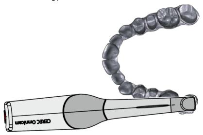
Position the camera occlusally above the last tooth on the right, to start the scanning process.
