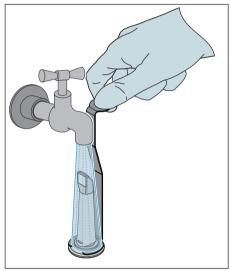
**12.** Carefully rinse the mirror sleeve with tap water for at least 30 seconds while holding it with the bracket.
