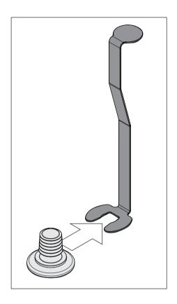
6. Push the plug completely into the metal bracket.
