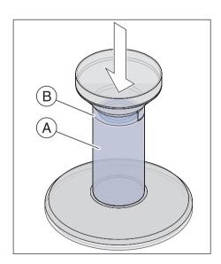
8. Carefully fill the HLD container up to the marking (B). You can use a funnel to pour in the fluid (A). Do not spill any disinfectant. Observe the safety instructions from the disinfectant manufacturer when cleaning if you do spill any disinfectant.
