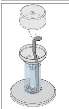
10. Place the cover on the container and leave the mirror sleeve in the disinfectant for at least 12 minutes (CIDEX®OPA). The mirror sleeve will not be damaged if it remains in the disinfectant for longer than the required time, but removing it shortly after the required time is recommended.
