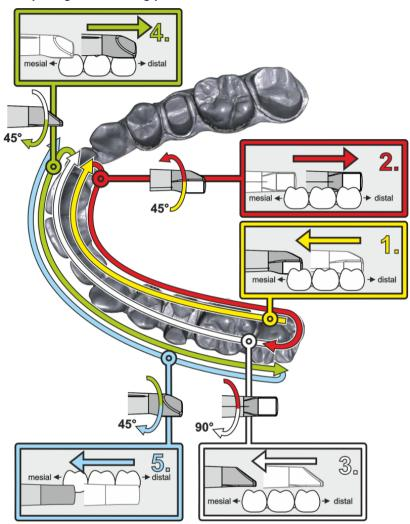
1. Start as indicated above, on the occlusal surface of the right terminal tooth, and scan it occlusally.
