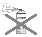
Do not spray liquids such as disinfectants into the ventilation slots. This may lead to malfunctions. Use wipe disinfection only in the vicinity of the ventilation slots.
