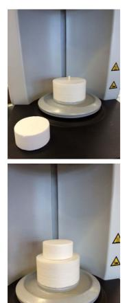
2. Start by placing the bottom door insulation on the positioning pin.
