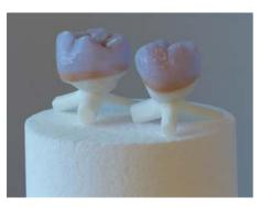
**4.** After this, position the restoration centrally on the top door insulation and ensure that the holder or restoration do not protrude out from the door insulation; otherwise, these may collide with the furnace chamber.
