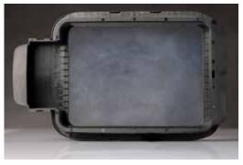
Prints or grease residues on the tank foil can be cleaned using isopropanol. The tank can then be used again.
