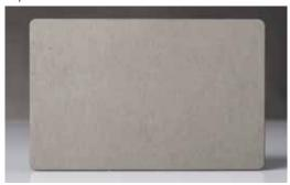
Minimal, insignificant scratches have no effect on the printing job and the build platform can still be used.
