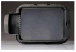
The material tank only needs to be replaced if there are deep scratches or holes, so that a completely flat tank surface is guaranteed. Superficial, light scratches in the film will not affect the printed result and the tank can be reused.
