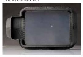
Raised surfaces or creases will change the surface tension of the foil. This can lead to problems in removing the object from the build platform and subsequently cause inaccurate results or misprints. Therefore, in this case, the tank should be exchanged. In addition, if there are deep cracks or perforations, the printing material can leak through the damaged area and contaminate the glass screen.
