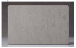
Deep scratches on the surface of the build platform make its surface rough. This can lead to damage to the tank foil when the build platform is immersed in the material tank at the beginning of the printing process. For this reason, if the build platform has deep scratches, it must be exchanged.
